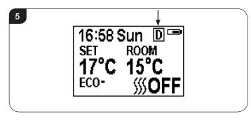
2b.11 Hold the ← button for 6 seconds to enter the daily heating setting. A maximum of 3 timed heating periods can be set per day.
