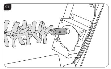
11.5 Withdraw the spindle from the left hand bracket, see Diagram 28. The spindle may need to be tilted to be removed from the location bracket.
