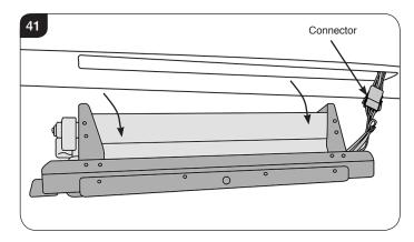
16.5 Carefully feed the wires over the between the Heater Assembly and Power Unit apertures.
