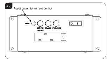
Resetting of the remote control is necessary if the appliance operates wrongly due to external interference signal and the remote control is not in use.
