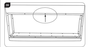
16.3 The Heater Assembly is now held in place by 5 screws at the top of the firebox. Supporting the Heater Assembly remove the screws, see Diagram 40.
