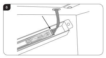
NOTE: When replacing the LED Light Bar ensure that the central tab is positioned at the front of the firebox.
