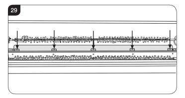
NOTE: When refitting the shield ensure that the lip curves down and towards the back. It will be necessary to lift the shield slightly to align the screws. Refit the screws from inside out. 12.3 The LED boards are located below the Effects Spindle, see Diagram 30.
